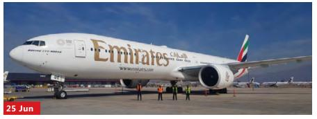
Emirates introduces the first of its 19 Boeing 777-300ER "mini freighters". These are passenger aircraft used to operate cargo missions with modified Economy class cabins that provide an additional 132m³ of cargo volume per flight.
